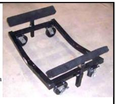
each have four heavy duty 6" x 2"phenolic resin caster wheels that swivel on ball bearings. Two of the dolly wheels have locking mechanisms. The dollies can be shipped by UPS. For safety reasons, dollies must be used in pairs.
