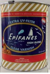
25%, the third coat 15%, and additional coats anywhere from 0 to 7%. [If you used sealer, thin your first coat 25%.] Do not thin your last one or two coats. Apply 12 to 14 coats for base coats, then every year or two, add two coats to maintain your ultraviolet protection, as this protectant is used up by exposure to the sun. You need at least 12 coats to get good u.v. protection. If you try to get by with fewer coats, you may have lifting and flaking after one summer in the sun.
