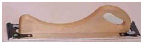
with Dayco Marine Stripper and a scraper. Then get the remaining stain out of the grain with a brass bristle pot scrubber brush [available at most grocery stores] and more Dayco Stripper. Do not begin sanding until the wood is completely clean. Start sanding with 80 grit paper and finish with 100 grit. Finer paper will not leave enough texture to fill with filler stain. 3M Gold Resin Bond Aluminum Oxide Paper is a very high quality sandpaper that outlasts other sandpapers and resists loading.
